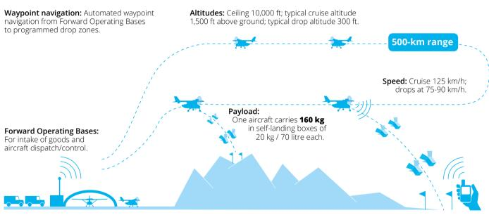
**Communication:** Direct radio control for take-off and landing; during flight, the aircraft are operated BVLOS by radio/satcom combinations, depending on the terrain and the required range.
